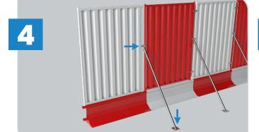
Secure the panels in place using a HD coupler at a height of 1.5m from the ground. Using the same coupler bolt attach the stabiliser as shown, the base of the stabiliser should be attached to the ground using chemical anchors of at least M12 x 110mm.
